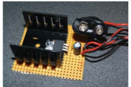
■ This is the power regulator to reduce the battery voltage to 5V for the Pi
