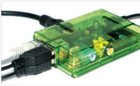
■ Fig 1: The Pi is ready to use with connections to peripherals, a monitor and the OS installed on an SD card
