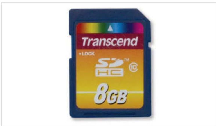
■ This is an SD card – it's your Raspberry Pi's boot and storage device, though you can add more with a USB drive
