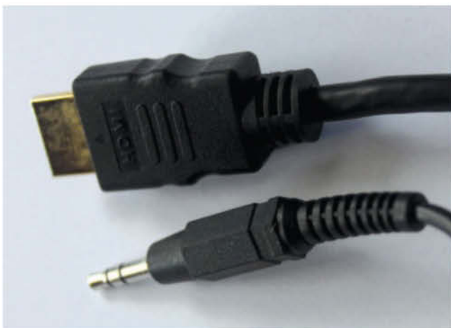
■ The cable at the bottom is a standard 3.5mm audio jack; above it is an HDMI cable. You can use either to output Pi audio
