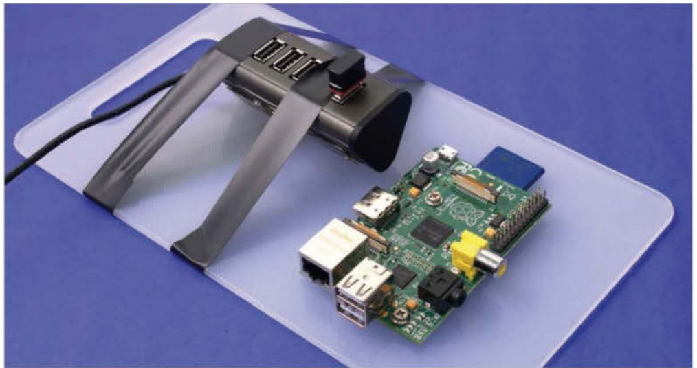
■ The Raspberry Pi with SD card and the powered USB hub fastened in position, ready to go into the folder
