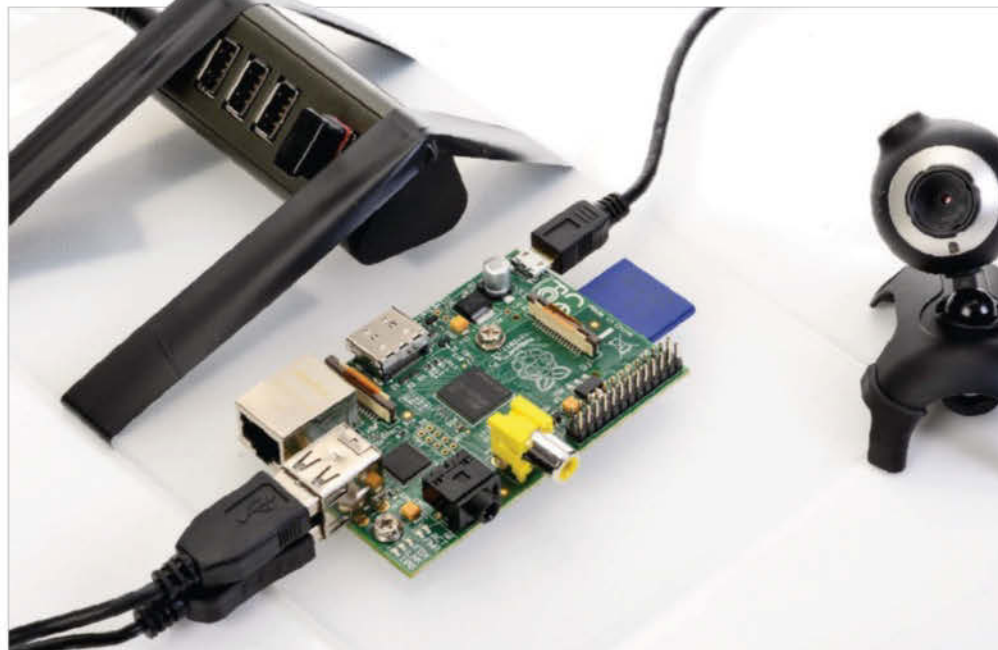
■ It may look complex but building a webcam server with your Raspberry Pi is easier than it looks (p. 84)
