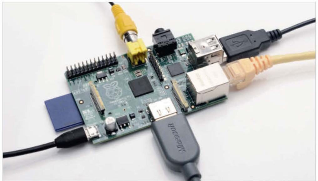
■ An operational Raspberry Pi - with USB, ethernet, HDMI, micro-USB and video out ports in use. One or more of these will be connected, depending on what you're using your Pi for
